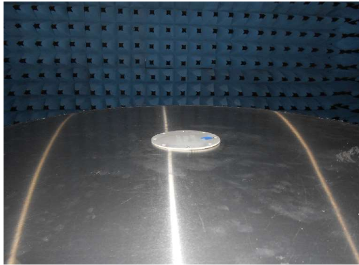
Figure 8-2: Horn Antenna Mounted on Curved Ground Plane
