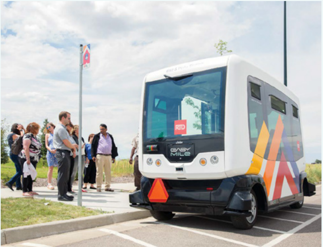
Circling the Panasonic and Peña Station parking lots, an autonomous shuttle is making history daily. The first on-road deployment of an autonomous vehicle shuttle in the state of Colorado, the shuttle is 100 percent electric and navigates a one-mile loop every fifteen minutes.
