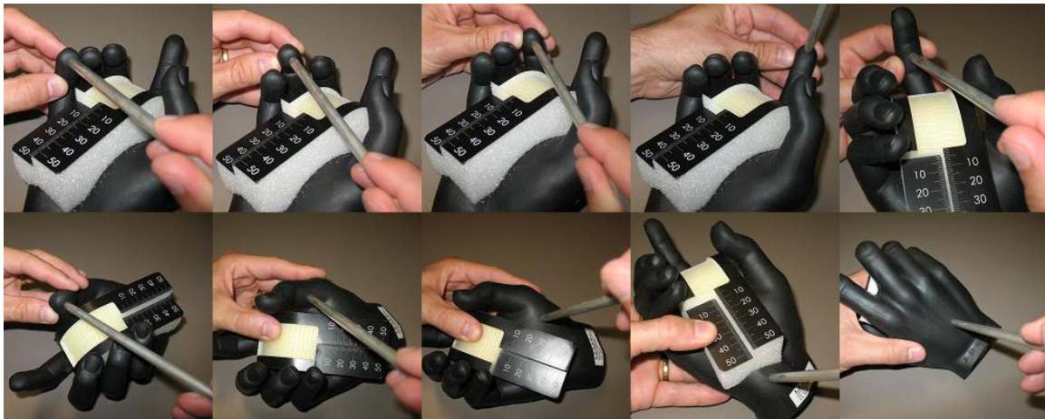
FIGURE G-2 THE TEN LOCATIONS OF DIELECTRIC MEASUREMENTS AT THE FOLD HAND SURFACE
